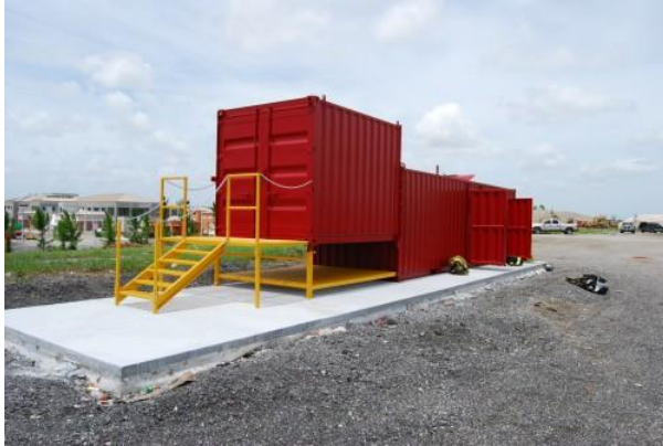
Figure 10 -- Swedish flashover simulator prop (typical)
