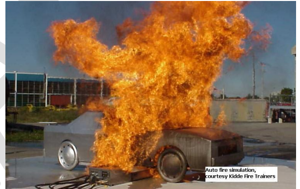
Figure 9—Gas-Fueled Vehicle Fire Prop
